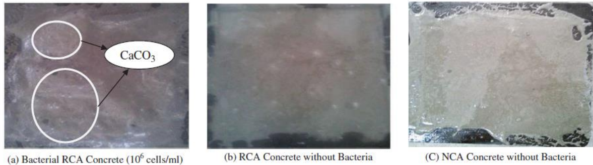
Fig 6 Pictures of new concrete showing rain calcium carbonate.
