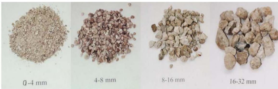
Fig 3. Shape and surface texture of different fractions of recycled aggregate
