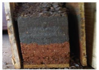
Fig. 9: Plate 8 – Merging - Improper Separation of sub-grade from the sub-base
