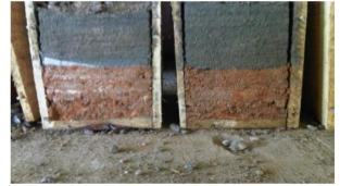
Fig 8: Plate 7 – Proper Separation of sub-grade from the sub-base
