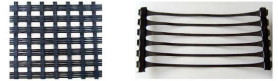
Fig. 2: (a) Biaxial woven geogrid and (b) Uniaxial geogrid
