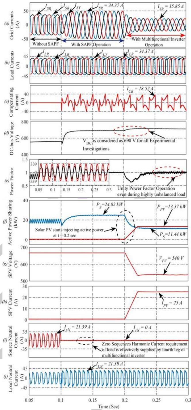
Fig. 4 System response under unbalanced loading: (a) Grid currents, (b) Load currents, (c) Compensating current, (d) DC-bus voltage, (e) Power factor, (f) Active power sharing, (g) SPV voltage, (h) SPV current, (i) Source neutral current, and (j) Load neutral current.
