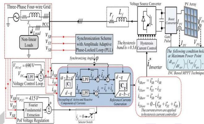
Fig. 2 Control algorithm to generate the reference currents
