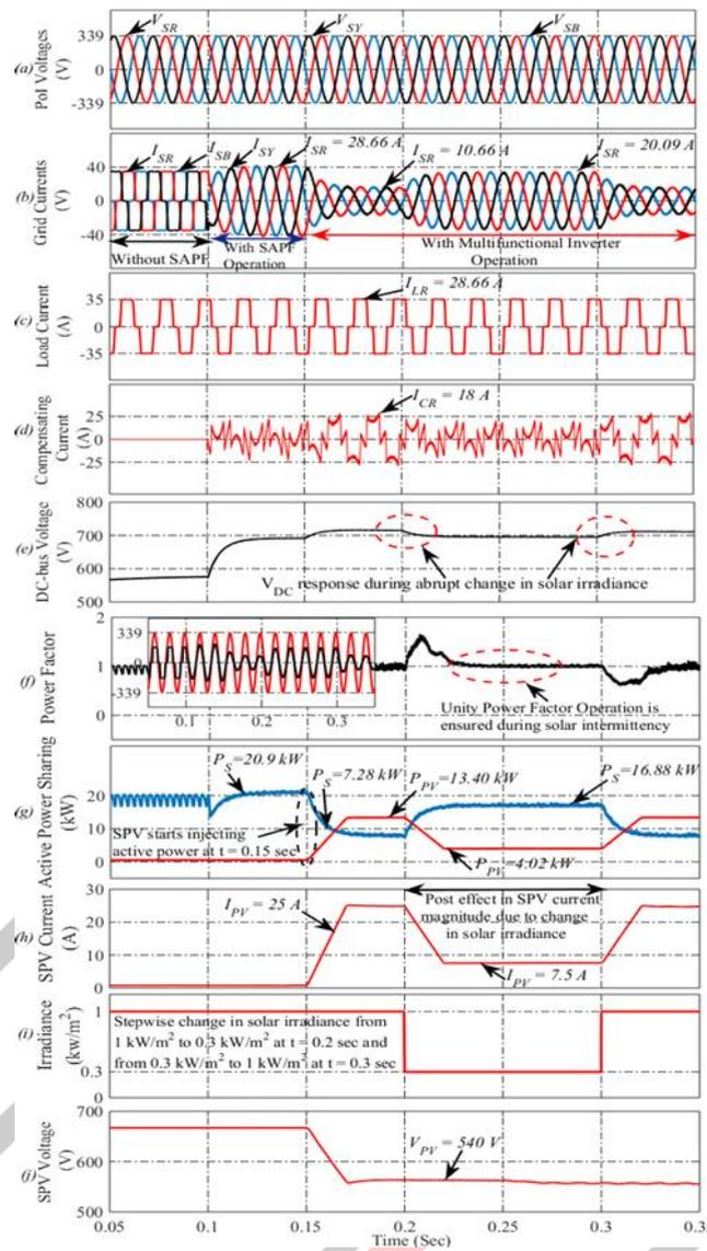
Fig. 5 System behavior under solar irradiation change: (a) PoI voltages, (b) Grid currents, (c) Load currents, (d) Compensating current, (e) DC-bus voltage, (f) Power factor, (g) Active power sharing, (h) SPV Currents (i) Solar irradiance, and (j) SPV voltage.
