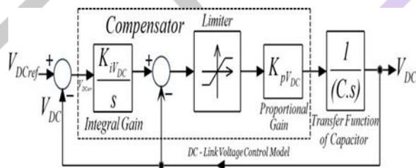
Fig. 3 Closed-loop control of the DC-bus voltage regulator
