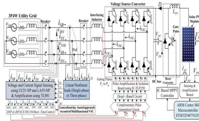
Fig. 1 System architecture for the grid-connected SPV system
