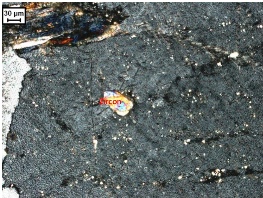
Figure 5: Zircon grain embedded in plagioclase feldspar, granodiorite of TGM Suite under crossed polar.
