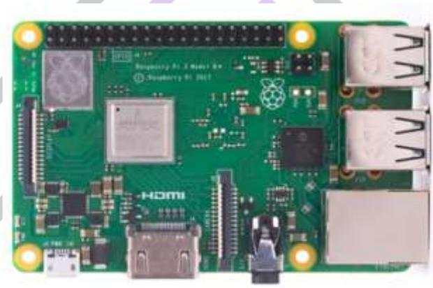
Raspberry Pi is a low cost, credit-card sized computer that plugs into a computer monitor or TV, and uses a standard keyboard and mouse. It is a capable little device that enables people of all ages to explore computing, and to learn how to program in languages like Scratch and Python.
