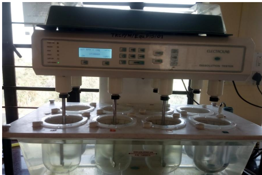
Fig 8.16 In vitro dissolution test apparatus
