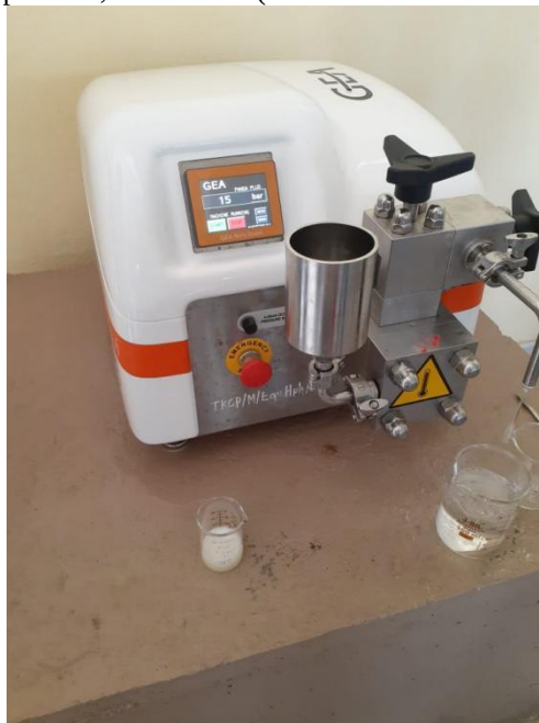
Fig 8.7 Preparation of OXZ polymeric nanosuspension
