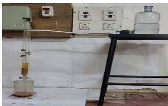
Figure 1: Pictorial view of column chromatography
