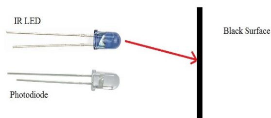
Fig.1.a IR sensors Reflection on black surface.
