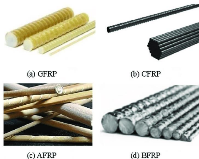
Figure 1 Four Different Forms of FRP Composites [6]
