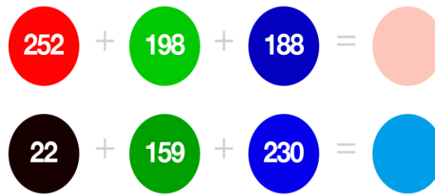
Figure 3.4: Top: A possible application for a skin detection programme involves combining different Red, Green, and Blue colour components to generate a "caucasian flesh tone."
