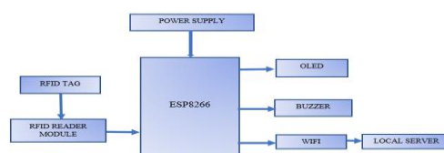
Fig 1: Smart cart billing system
