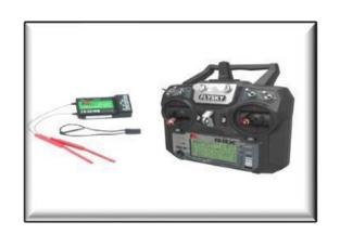
The radio control system consists of two corridor, a handheld transmitter and a receiver that attaches to your drone. Keeping effects simple then, your drone will read your stick input and shoot it through the air to a near receiver. Once the receiver has this information, a drone regulator is transferred, which in turn operates the drone.
