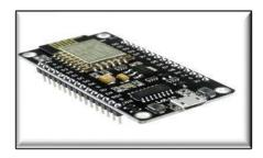
The "Smart Irrigation Systems" electrical college project uses a NODEMCU board to improve the project's efficacy and efficiency. The ESP8266 Wi-Fi module serves as the foundation for the open-source NODEMCU Internet of Things platform. This low-cost, low-power, and fully integrated microcontroller board may be used to create a variety of applications. It is an excellent choice for activities needing wireless communication, such as a smart irrigation system.
