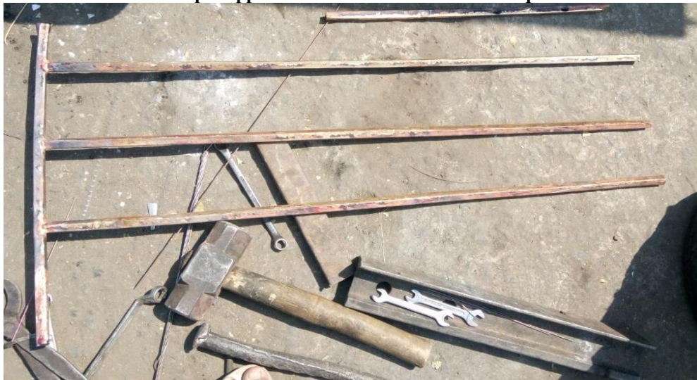
Plate 3 Assembly of Solar water Heater Pipe
