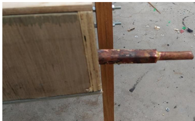
Plate 4 End Connection of Solar Water Heater
