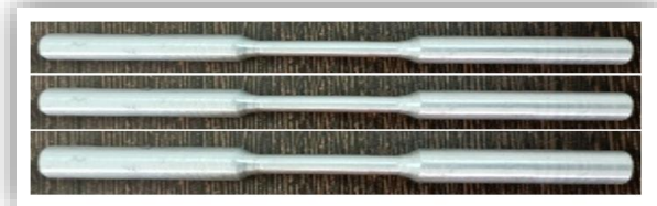
Fig 4 Tensile test specimen
