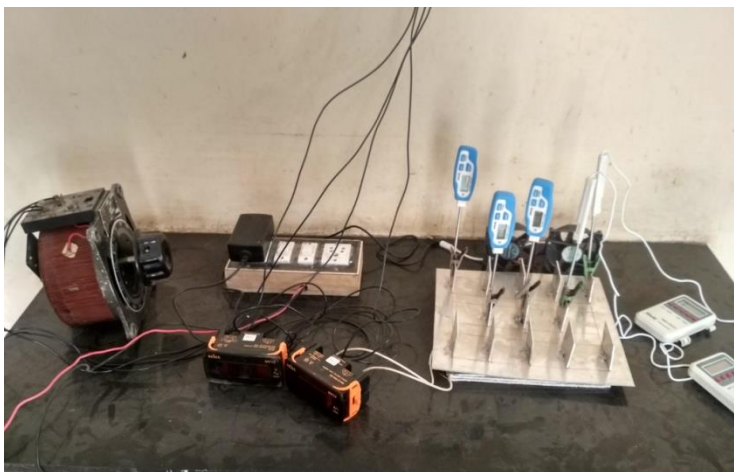
Fig.4: Actual Experimental Set Up of Parallel Split Fin Pattern
