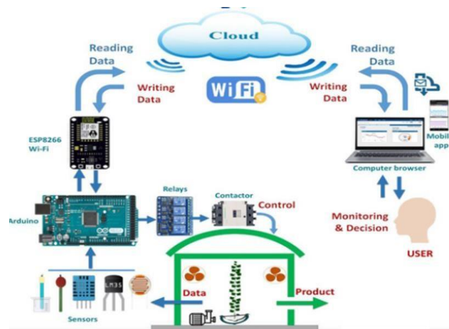
Figure 2: Overall schematic diagram of an IoT-based monitoring system for crop parameters
