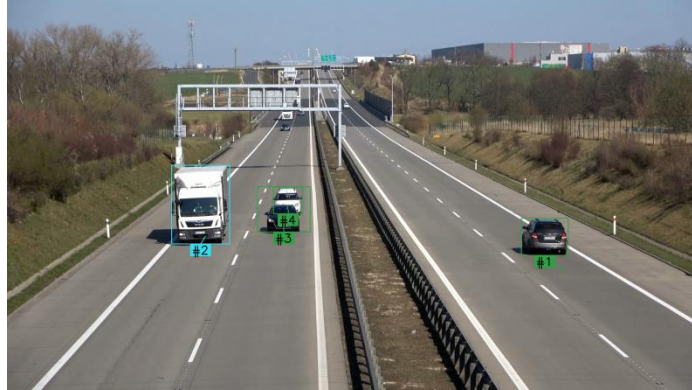
Figure 3. Screenshot of Traffic Video Analysis: Vehicles on Road with Vehicle Count Annotations
