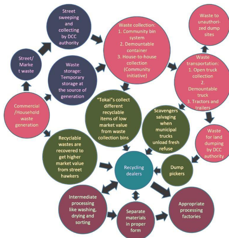
Fig. 2 Existing waste management systems' flow [6]
