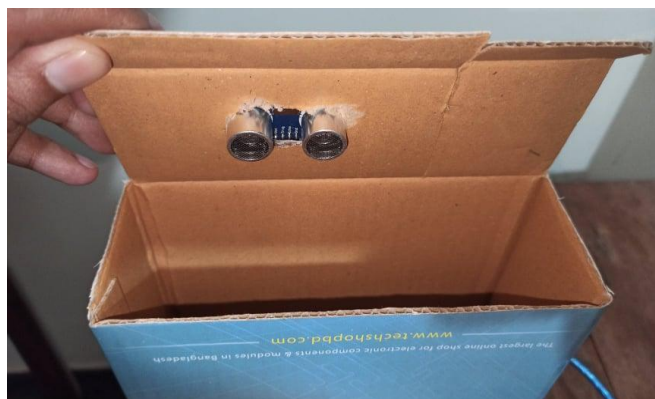
Fig. 6 Implementation of the sensor in a dump bin (Demo)
