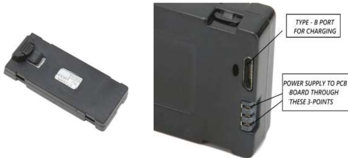
Figure 4. DC 3.7 Volts (1800 Mah) Battery.
