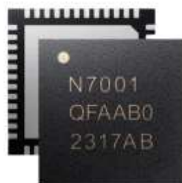
Figure 3. nRF7001 IC of the Drone.
